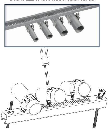
To install, insert the tabs of the Smart-Clamp into the slots
