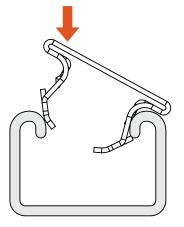
1. Place one side of the locking tab into strut channel
